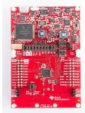
SimpleLink™ CC26x2R LaunchPad™ Development Kit
